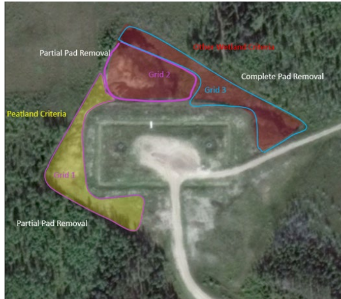
Figure 2: Diagram of the three grids surveyed in 2018. The yellow area passed the peatland criteria while alternative wetland criteria are recommended for red areas.
