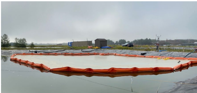
Figure 2 – SolarPass FRB scale-up module utilized for testing deployment, containment, environmental factors, and collection at InnoTech Alberta’s Vegreville demonstration lagoon.
