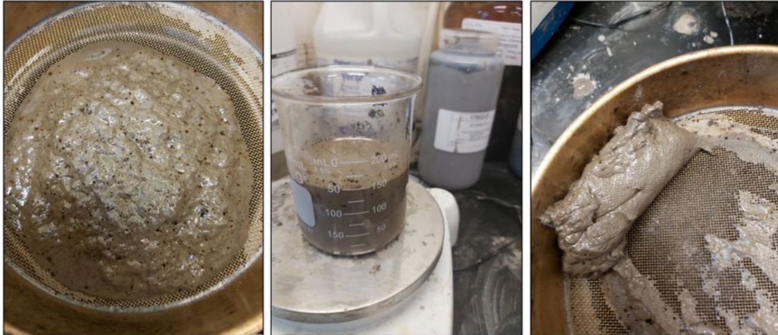
Figure 2: MFT Flocculation Test using Suncor Test Method
